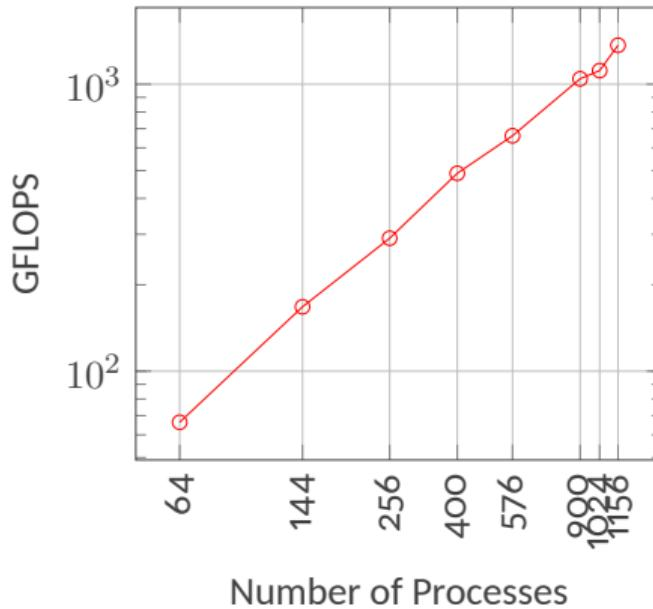
We can see that the time remains roughly constant as we increase the number of processes, while the performance increases accordingly  $N =$ ,  $NB =$ .
